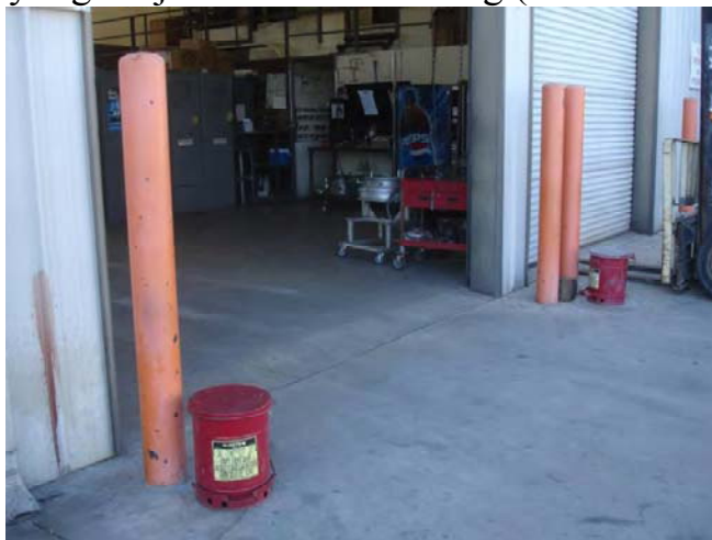
d. Bucket for oily rags adjacent to the building (225 West Slover Avenue).
