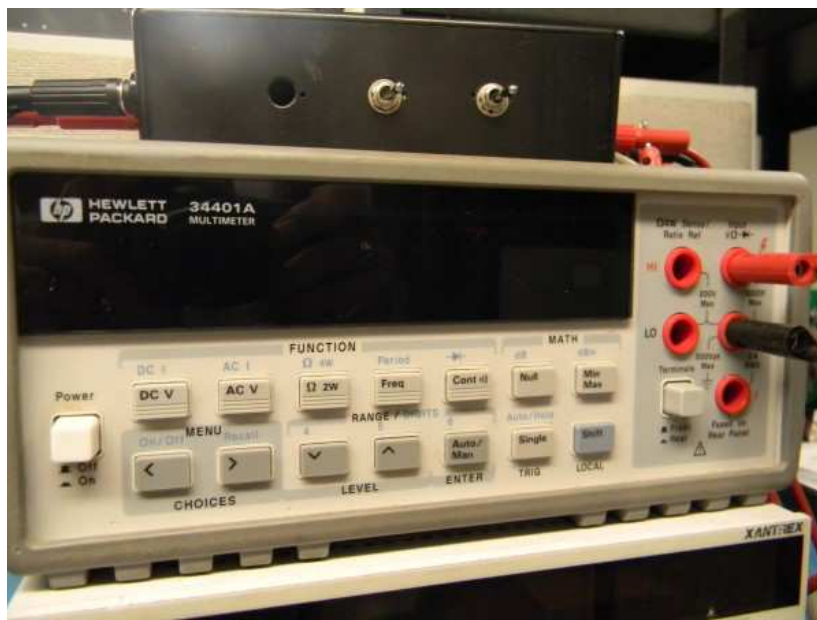
HEWLETT PACKARD MULTIMETER MODEL 34401A, S/N US36055120
