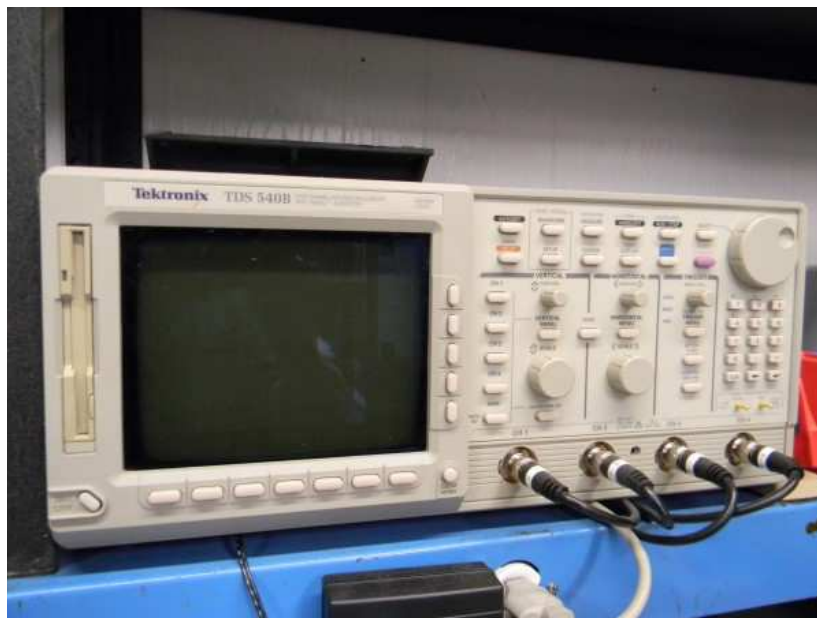
TEKTRONIX FOUR CHANNEL DIGITIZING OSCILLOSCOPE MODEL TDS-540B S/N B020692, W/ INSTAVU, 500 MHZ, 2 GS/S
