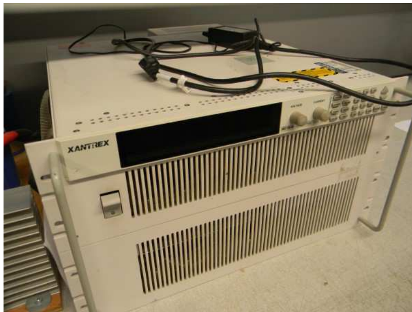
XANTREX DIGITAL DC POWER SUPPLY MODEL XDC150-80, S/N E00084545, 0-150V, 0-80A
