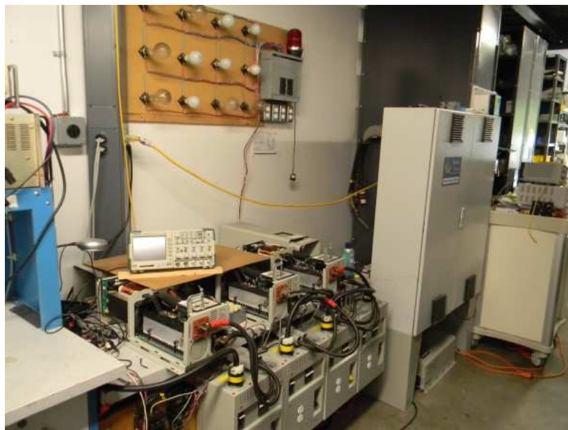
CUSTOM SHOP MADE TEST BENCH FOR APOLLOS SOLAR 4048V INVERTERS, (16) 12 VOLT AUTO BATTERY POWERED, CABINET
