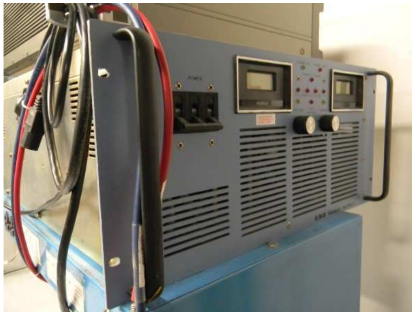
LAMBDA ESS HIGH POWER DC POWER SUPPLY MODEL ESS400-25-2-D-RSTL, S/N 21A2480 400 VOLT, 25 AMP
