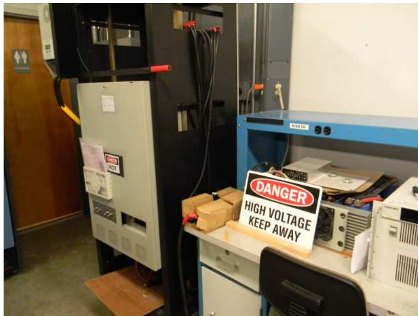
CUSTOM SHOP MADE TEST BENCH FOR APOLLO CHARGER CONTROLLER, HIGH VOLTAGE POWER SUPPLY
