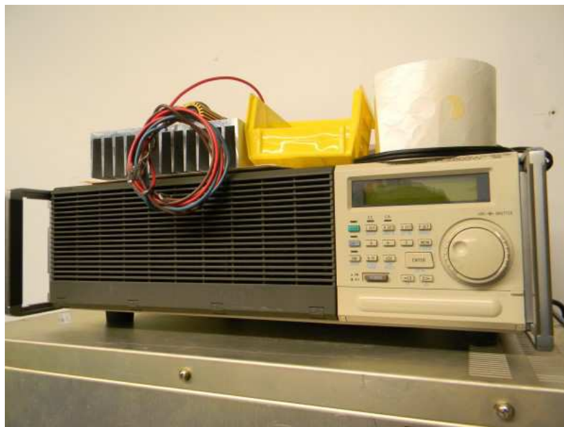
KIKUSUI ELECTRONIC LOAD MODEL PLZ603W, S/N 1100026, 1.5-120V/0-20A, 600 W
