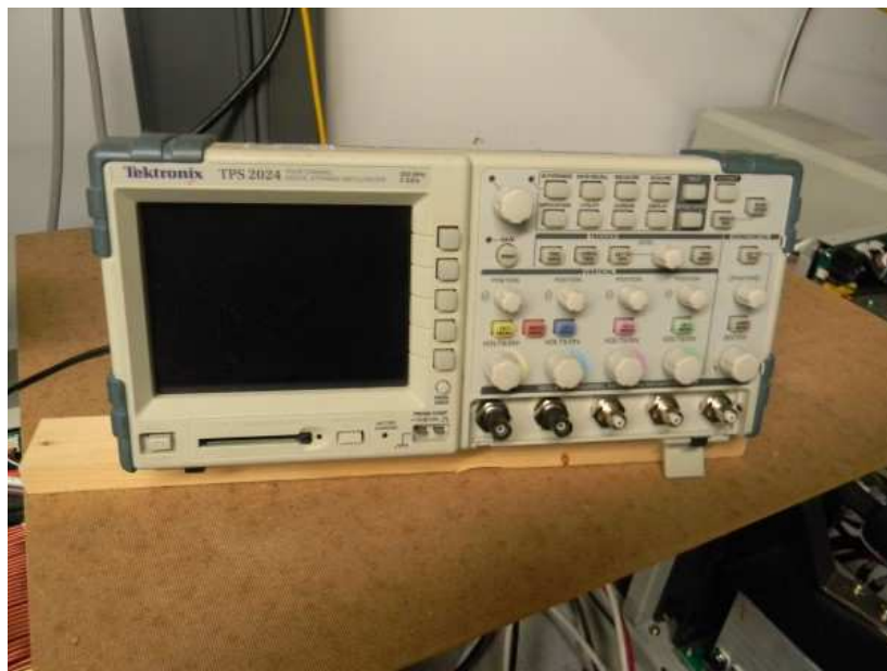
TEKTRONIX FOUR CHANNEL DIGITAL STORAGE OSCILLOSCOPE MODEL TPS2024, S/N C010371, 200 MHZ, 2 GS/S
