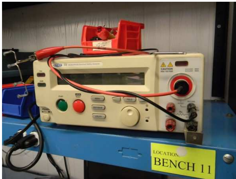
VITREK AC/DC/IR/GB HIGH ELECTRICAL SAFETY ANALYZER MODEL V4, S/N 16688, 6.0 KVDC MAX
