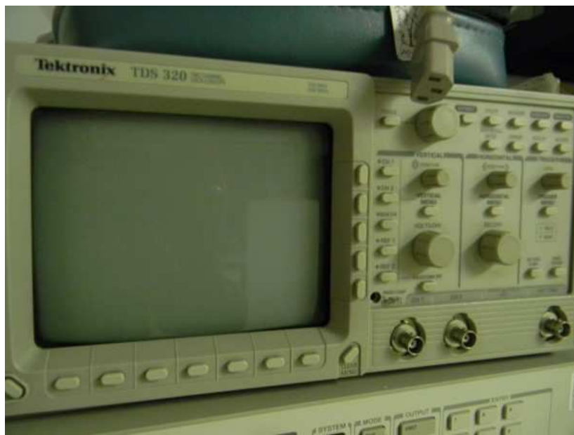
TEKTRONIX TWO CHANNEL OSCILLOSCOPE MODEL TDS320, S/N B033318
