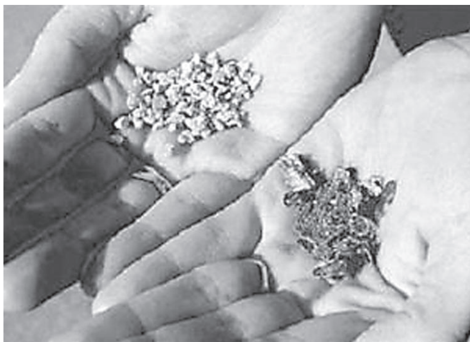
Figure 3: Raw (Right) and Popped (Left) Vermiculite
