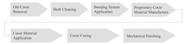
The covering on the rolls used in the paper-making process wear over time and must be periodically replaced for the roll to function properly. Rolls are removed from the paper-making machine and taken to an offsite facility for re-covering. During this time, a spare roll is placed in the machine to enable continuous operations.
