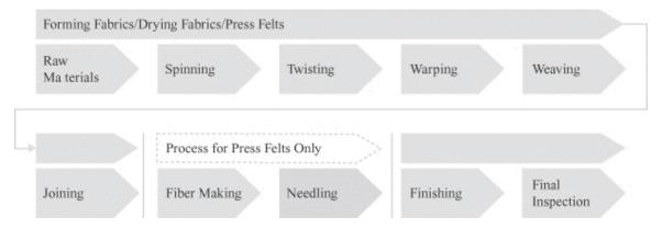
The clothing production process begins with the spinning of synthetic fiber threads to produce yarn, which is then twisted in preparation for the manufacturing of clothing. Yarn, which is sometimes purchased as a raw material, is then wound on large spools prior to installation on the loom. The yarn is drawn through needles in preparation for weaving.
